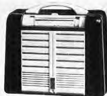
The appearance of the Bush BP10 portable. The scale cover (shown open) operates the battery switch.
