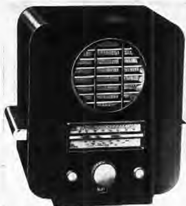
The Ekco B74 superhet in the black and chromium cabinet. The seven-barred speaker grill is removable.
